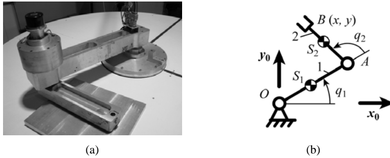
Figure 2. The 2R serial robot: (a) prototype; (b) schematics.
